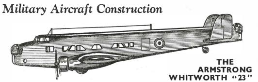
DESIGNED to combine the duties of long-range bombing and troop transportation, the Armstrong Whitworth Type 23 is one of the latest bomber-transports to be built for the Royal Air Force. A twin-engined, low-wing cantilever monoplane, it has an unusually roomy cabin for the transport of troops, supplies, spare engines, etc., and is fitted with an undercarriage that can be withdrawn into the engine nacelles. The gunners' cockpits
